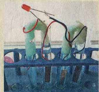
A functional electrochemical cell fabricated by Muskan Goyal, an IGCSE student, during a regular online chemistry class. The cell was made using zinc electrodes, copper electrodes, and zinc sulfate and copper sulfate solutions
